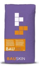
Mix one 20 kg bag with approximately 100-120 kg of dry graded aggregates 0-8 mm in diameter (1800 kg/m3) and approximately 12 Lt of water until a homogeneous mix is obtained. The amount of water could vary depending on the moisture in the aggregate.
